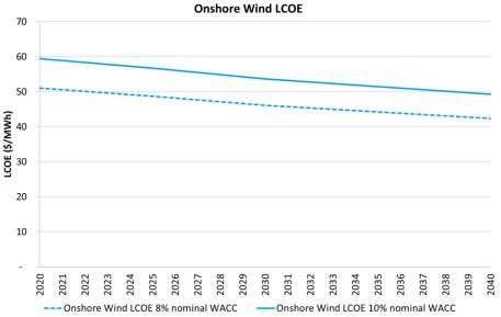
Figure 2: Indicative LCOE for onshore wind in the NEM, with and without a 2% WACC increase
