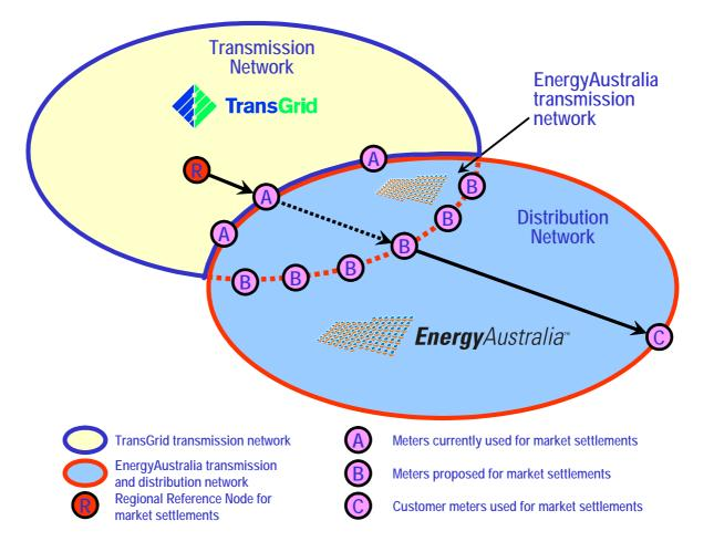
Consistent with the requirements of the Rules, EnergyAustralia has *metering installations* at the required connection points with other industry participants – transmission to transmission connection points with TransGrid and distribution to end customer connection points.
