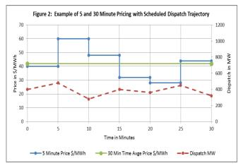
The figure shows the average price used for all energy generated in the half hour. The 5 minute price will typically vary above and below this average, which breaks the link between dispatch and potentially drives bad behaviour
