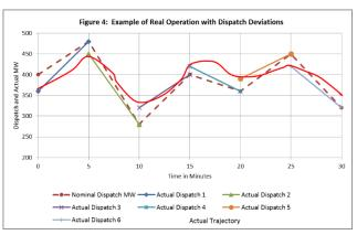
The idealised dispatch as discussed so far in this article is shown as the dashed line. However, the generator will never follow the trajectory exactly, as shown in the curved line. So the Initial MW for each 5 minute interval is never the exact MW in the previous schedule, but some deviation from it. However, at the 5 minute boundary AEMO re-sets the generator status to the actual MW as measured by
