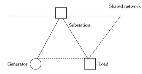
Assume in this example that the TNSP needs to reinforce the network serving the load for reliability reasons. It may be more efficient for the TNSP to build a new line from the generator direct to the load (the dashed line) rather than building a line to the load from elsewhere on the existing shared network (the dotted line).
