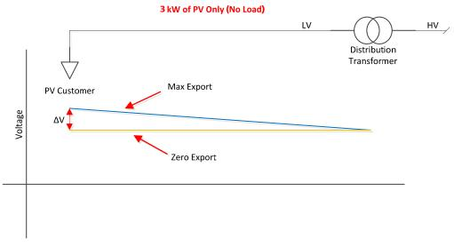
Figure 4: Premise with 3kW of PV (No Load) - Change in Voltage Profile
