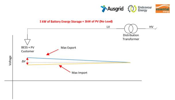
Figure 6: Premise with 1kW of Battery Energy Storage and 1kW of PV (No Load) - Change in Voltage Profile
