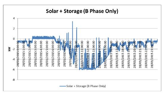
Figure 3: Example of Battery Storage and PV Controlled for Load Leveling
