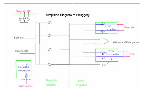
This simplified diagram shows the major connections at Snuggery substation. Connected at the substation are large generators (Lake Bonney and Synergen) and large embedded generator (Canunda), a large consumer (KCA) and a number of small consumers. Canunda exports more power than KCA and the other consumers guarantee to take at any time, indicating that Canunda needs access to the transmission system.
