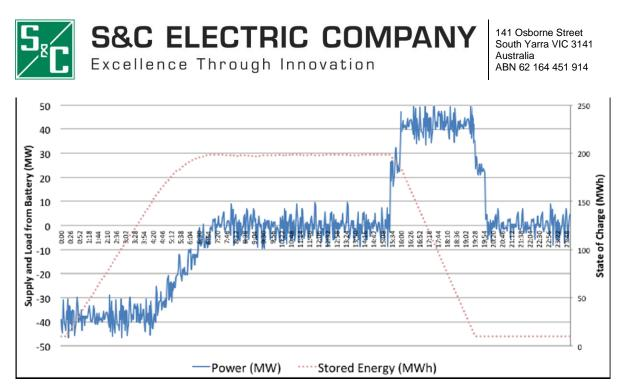
Battery continuously delivers frequency support, while charging and discharging (red dashed line) and delivers capacity from ~1600 to 1930.
