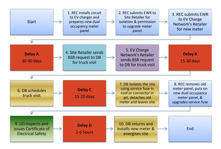
Figure 1 - Process for Establishing Separate Metering
