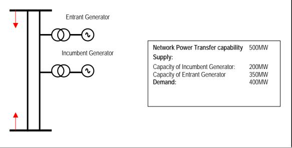
The example in Figure 3 depicts a situation where a connection applicant may request an augmentation because the power transfer capability of the network will be inadequate to enable all generators to operate at full capacity following the new connection.
