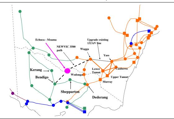
Note. 500kV lines (blue), 330kV lines (orange), 220kV lines (green), 275kV lines (purple),
