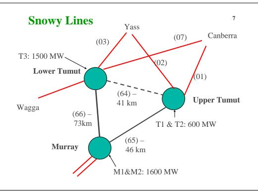
Note: Transmission line numbers are in brackets. The lines between Murray, Lower Tumut, and Upper Tumut are 330kV lines. M1 and M2 represent the Murray power stations and T1, T2, and T3 represent the Tumut power stations.
