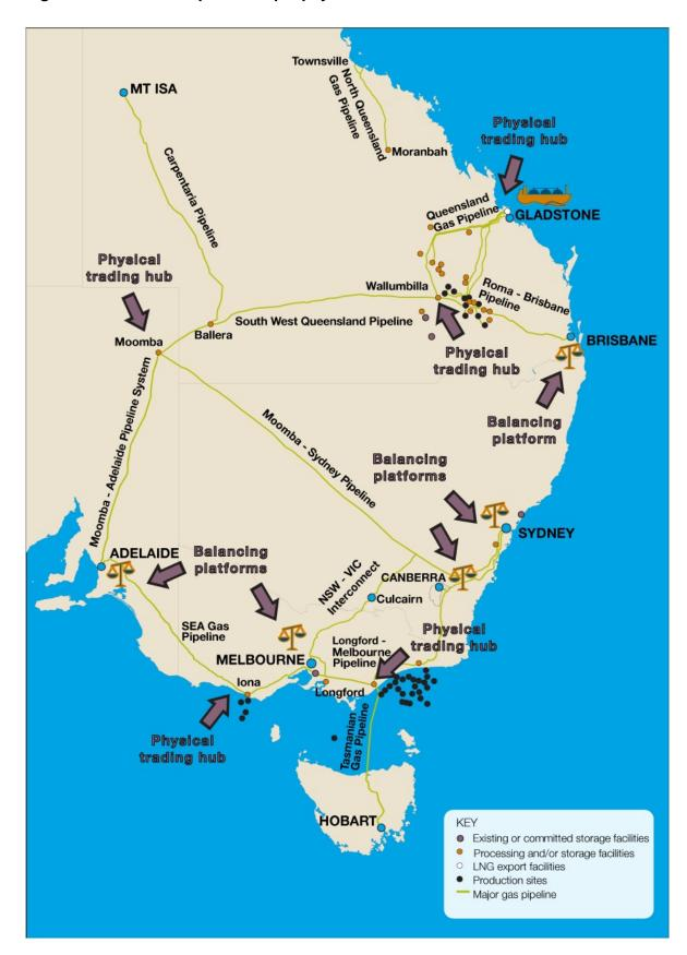
Figure 8.1 Concept 1: Multiple physical hub locations
