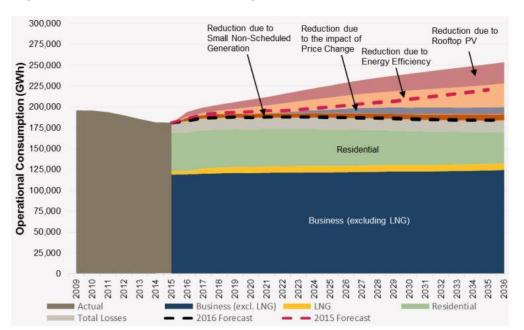
Figure 3.1 Forecast electricity consumption in the NEM
