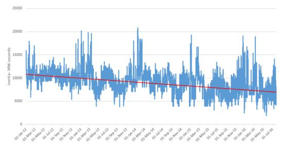
Figure 5.5 Inertia in South Australia
