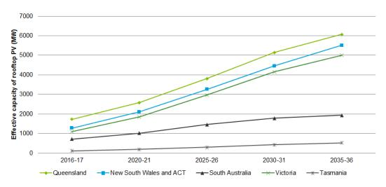
Figure 3.8 Installed rooftop PV capacity forecasts
