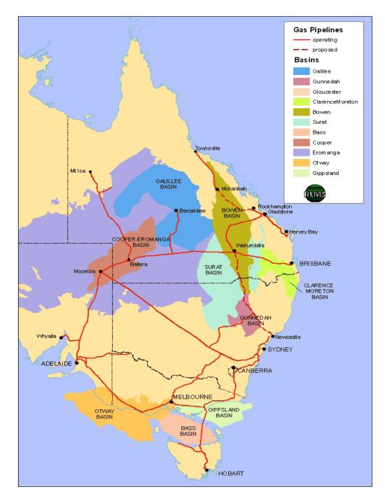
Figure A2: Existing and proposed gas transmission pipelines in eastern and southern Australia
