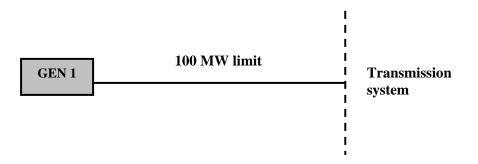
The constraint equation would be "formulated" by NEMMCO to ensure that the 100 MW limit on the line is not breached, i.e. that the output of generator GEN 1 does not exceed 100 MW. This constraint equation would therefore take the form:
