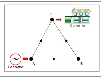
The flow of power across the network means that when a limit is reached on one part of the network, adjustments have to be made in generation and consumption across the network to ensure that the limit is not exceeded.
