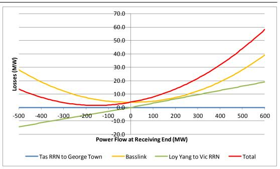
When Basslink is exporting 600 MW from Tasmania to Victoria, as measured at the receiving end at Loy Yang, the average losses based on the SNSP loss model are 58MW and the marginal losses are about 15% for the transfer from the Tasmanian RRN to the Victorian RRN.
