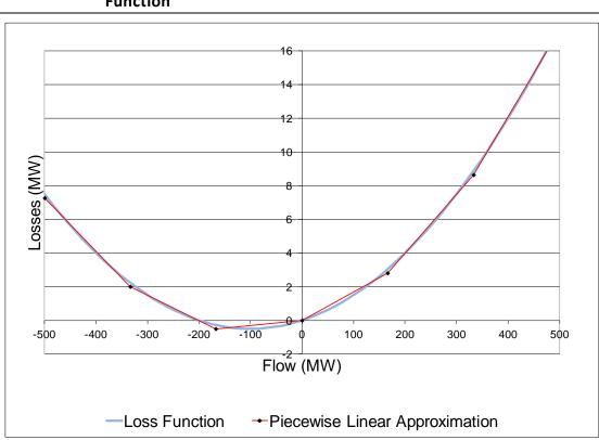
Figure 8 Example of Piecewise Linear Approximation of Quadratic Function
