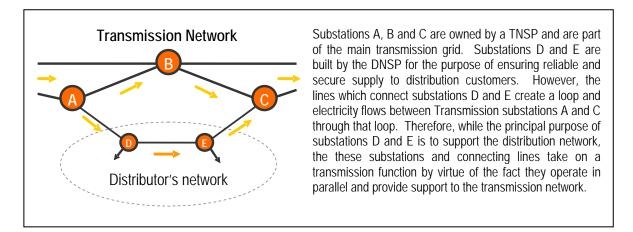
This is a simplified illustration of what can be a complex array of loop flows where transmission and distribution network assets meet at the margin. These instances are most common in urban and densely populated areas where the distributor's network is interconnected between higher voltage transmission substations to provide the required levels of security of supply to distribution customers.
