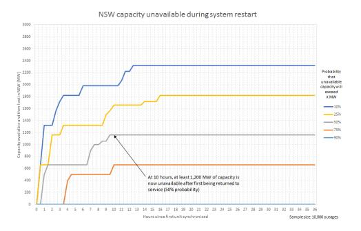
The graph shows by the hour the probability that generating capacity trips out after first being returned to service. For example, at the 10 hour mark there is a 50% probability that at least 1,200 MW of capacity that had been returned to service will no longer be running.
