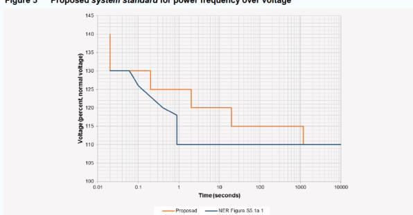
Figure 5 Proposed system standard for power frequency over voltage
