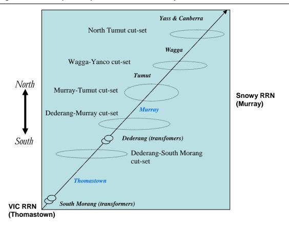
Figure D.4 Simplified representation of VIC-Snowy notional interconnector
