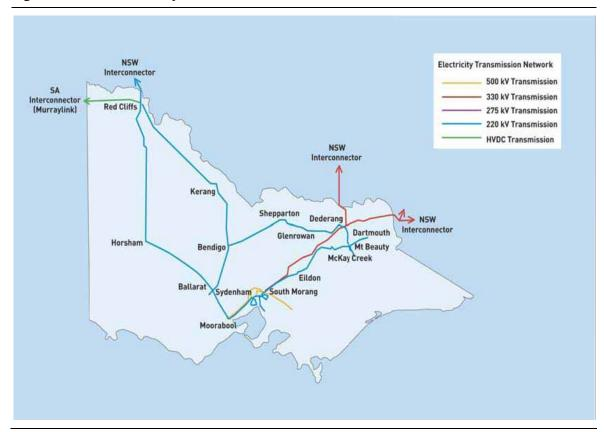
Figure D.5 VIC-Snowy – main transmission elements
