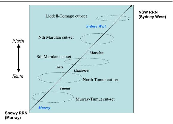
Figure D.2 Simplified representation of Snowy-NSW notional interconnector
