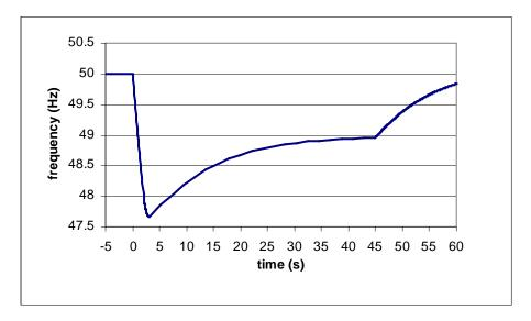
The operation of UFLS has been summarized in the following table. Estimated load of 25 MW has to be manually shed (simulated 45 seconds after the separation for the purpose of demonstration) to restore the frequency to 50Hz.
