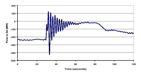
This type of response is required it shows a dynamic active power response from all units in the system. The settling is caused by the rotating masses settling into a new steady state equilibrium. The rules expect this type of response and the technical standards require the system to have a 5 second halving time. Without dynamic active power present in the power system in all areas, the system will suffer greater load shedding, and more severe power system disruptions.
