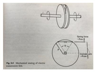
To use a spring constant analogy, we can represent the strength of a transmission line:
