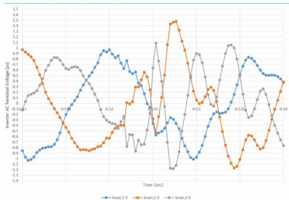
Figure 5.2: LV phase voltages during a transmission fault
