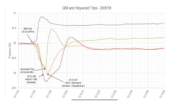
*Figure 2: Regional frequency during the separation events on* 25<sup>th</sup> *August 2018 (Figure 4 from AEMO Preliminary report: Queensland and South Australia separation on* 25<sup>th</sup> *August 2018 – published 7<sup>th</sup> September 2018).*
