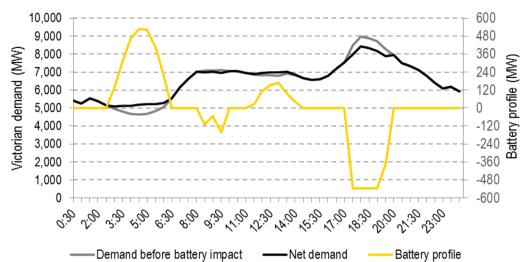
Figure 3: Example day of impact of behind-the-meter battery storage in Victoria
