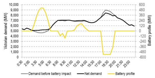
Figure 22: Example day showing impact of behind-the-meter battery storage on operational demand in Victoria
