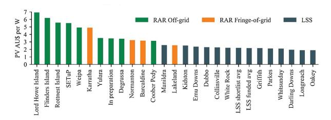
Figure 2 - PV \$/Watt for ARENA off-grid, fringe-of-grid and on-grid (Large Scale Solar) projects<sup>3</sup>
