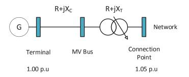
As the voltage of the MV collector system may return to within the maximum threshold limits of 85% to 112% prior to the *connection point* being restored to 90% to 110%, the only mechanism to sustain a reactive response in accordance with S5.2.5.5 is via a PPC which has visibility of the *connection point* voltage. TasNetworks considers it is important that this fact be clearly communicated in the AEMC's final determination.
